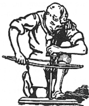
The Red Indian and Scout method of fire-lighting uses bow and drill.
